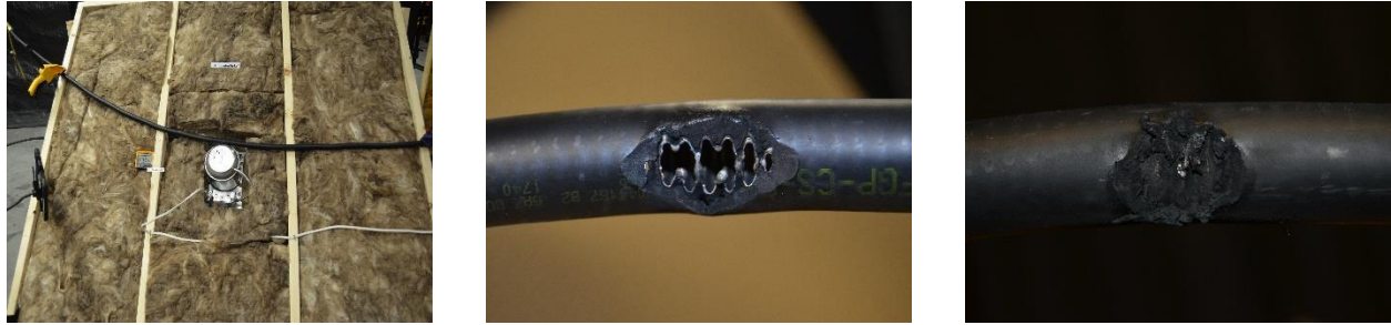
Figure 25 Test series 3 in place (left). Range of damage incurred to CounterStrike® CSST across test series 3 (center & right).
