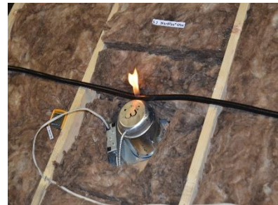
Figure 60 Fire resulting from test 5.3.
