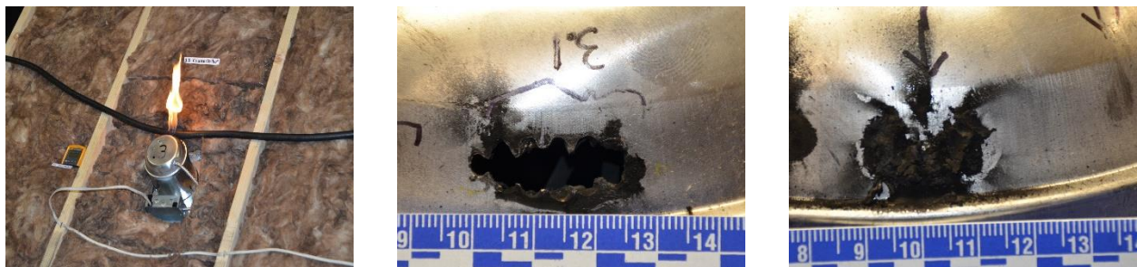
Figure 26 Example of fire resulting during test series 3 (left). Range of damage incurred to light fixtures across test series 3 (center & right).
