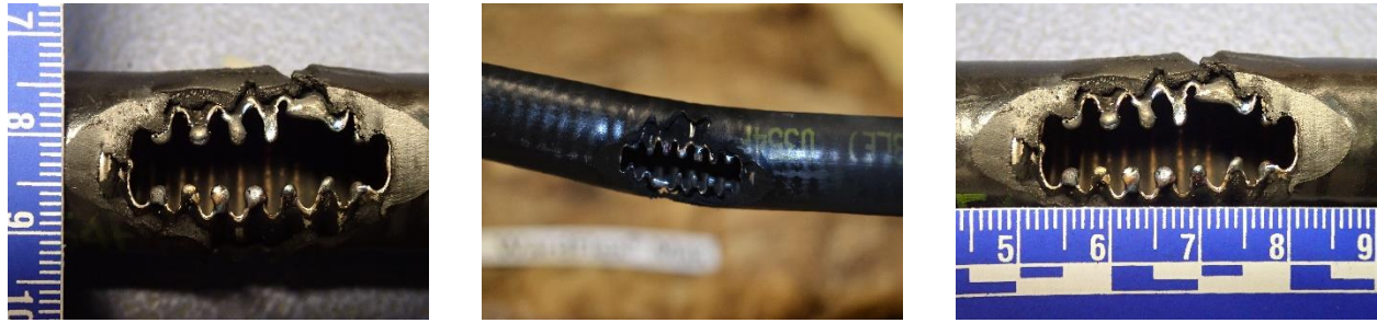
Figure 54 Damage to WARDFlex® Max CSST in test 5.2.
