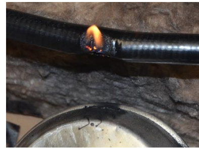
Figure 50 WARDFlex® Max CSST outer jacket burning without gas.
