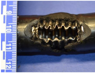
Figure 58 Damage to WARDFlex® Max CSST in test 5.3.
