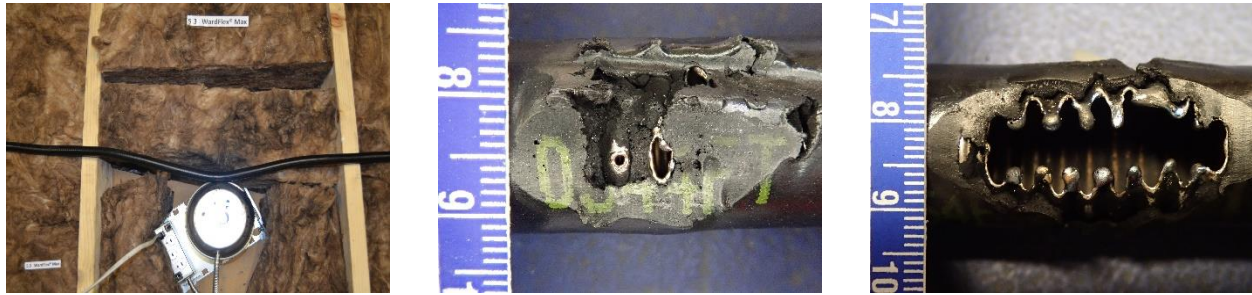
Figure 48 Test series 5 in place (left). Range of damage to WARDFlex® Max CSST in series 5 testing (center & right).
