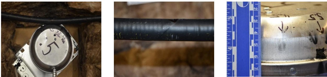
Figure 47 Test 4.5 in place (left). Undamaged FlashShield™ (center) & light fixture (right) post-test.
