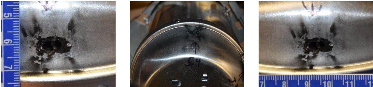
Figure 63 Damage to light fixture in test 5.4.
