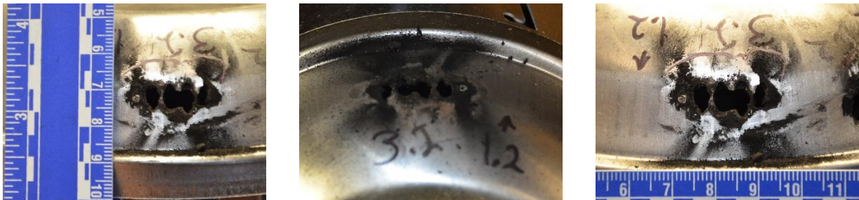
Figure 31 Damage to light fixture in test 3.2.
