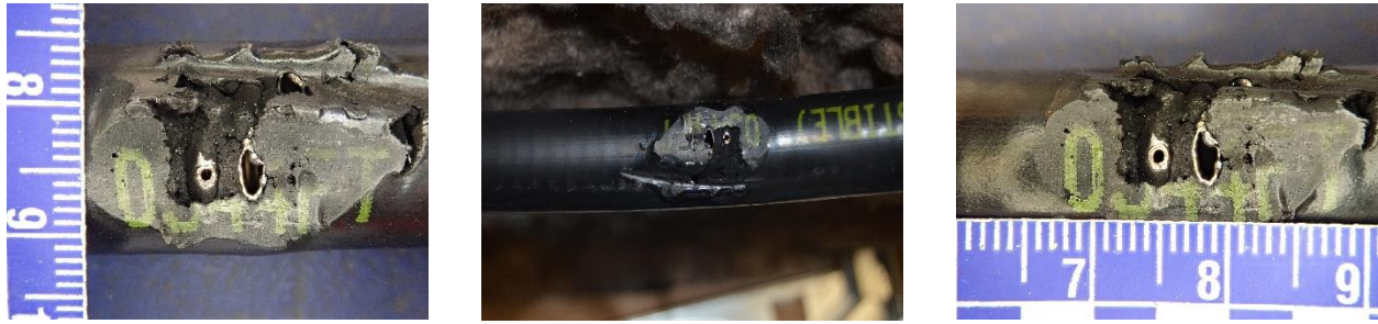
Figure 65 Damage to WARDFlex® Max CSST in test 5.5.
