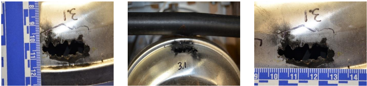
Figure 28 Damage to light fixture in test 3.1.
