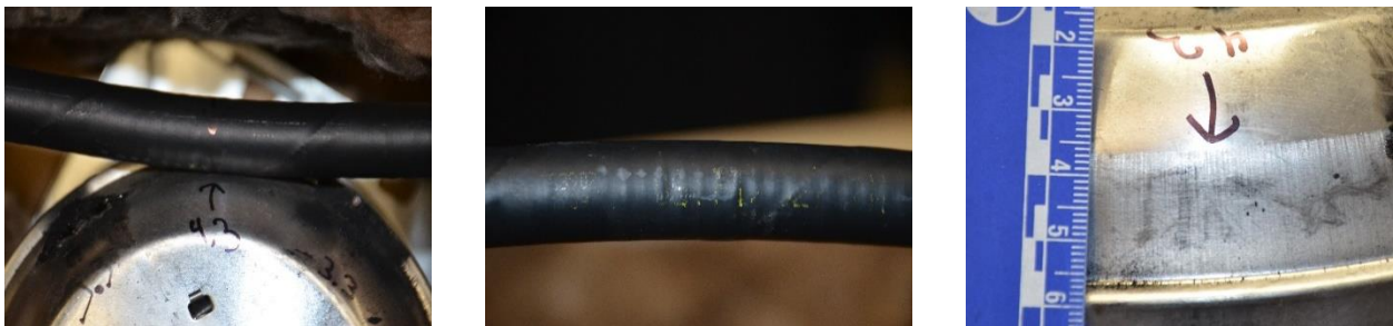
Figure 45 Test 4.3 in place (left). Undamaged FlashShield™ (center) & light fixture (right) post-test.
