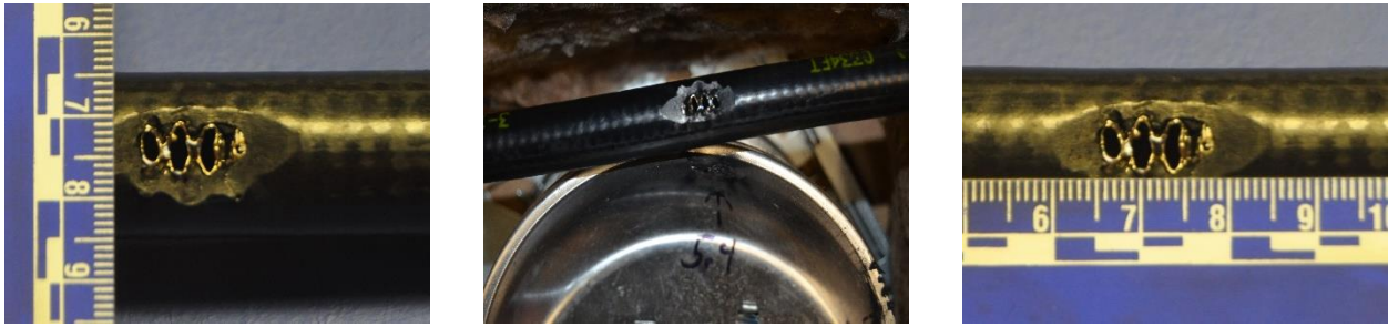
Figure 62 Damage to WARDFlex® Max CSST in test 5.4.
