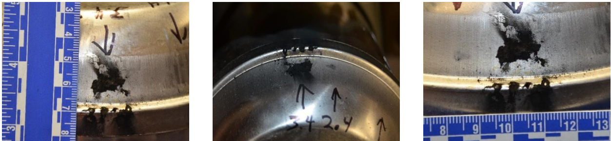
Figure 37 Damage to light fixture in test 3.4.
