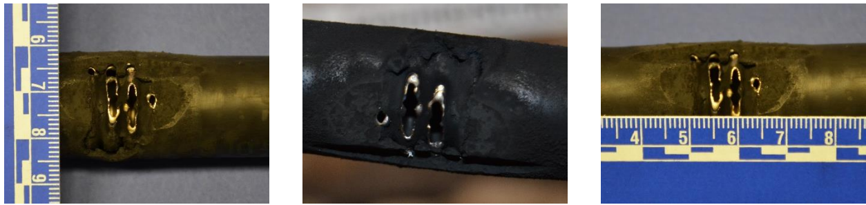
Figure 33 Damage to CounterStrike® CSST in test 3.3.
