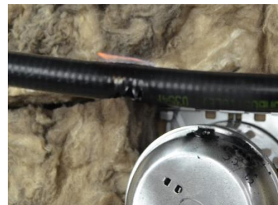
Figure 57 WARDFlex® Max outer jacket burning with gas turned off.
