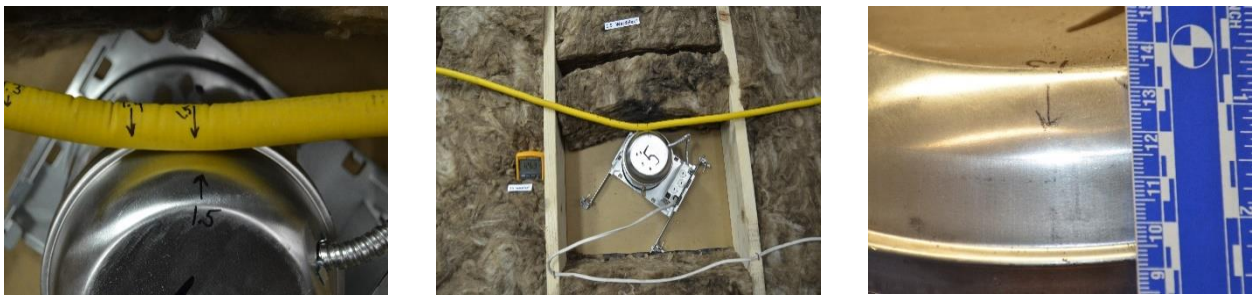
Figure 16 Test 1.5 in place (left & center). Undamaged light fixture post-test (right).
