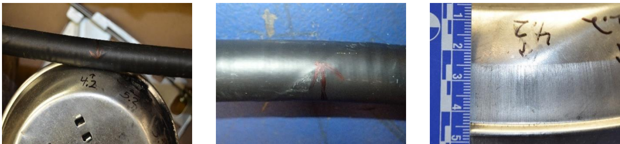
Figure 44 Test 4.2 in place (left). Undamaged FlashShield™ (center) & light fixture (right) post-test.
