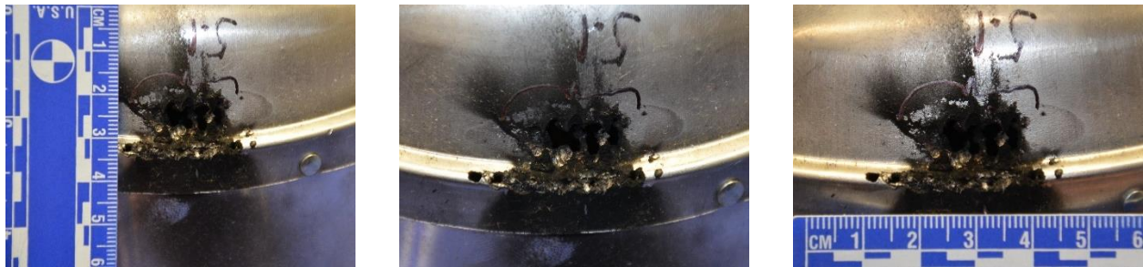
Figure 52 Damage to light fixture in test 5.1.
