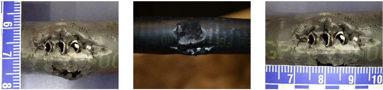
Figure 36 Damage to CounterStrike® CSST in test 3.4.
