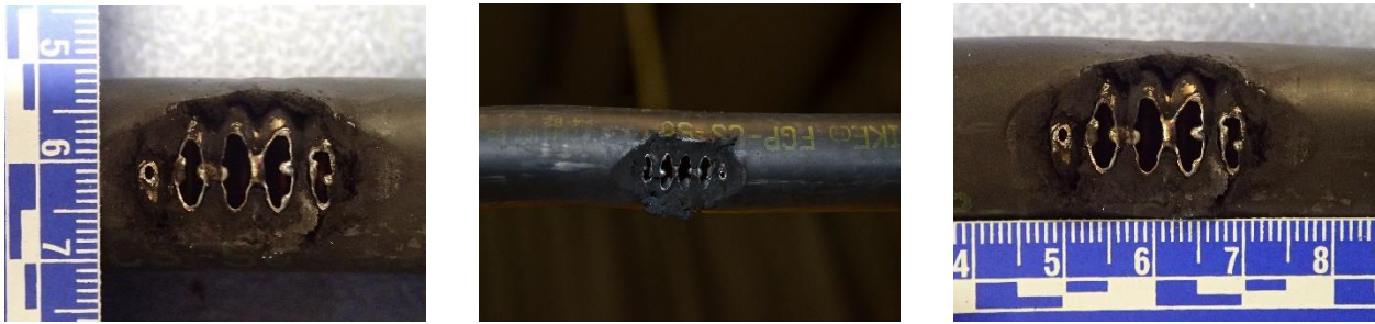
Figure 30 Damage to CounterStrike® CSST in test 3.2.
