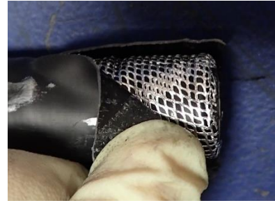
Figure 41 FlashShield™ CSST aluminum mesh layer visible.
