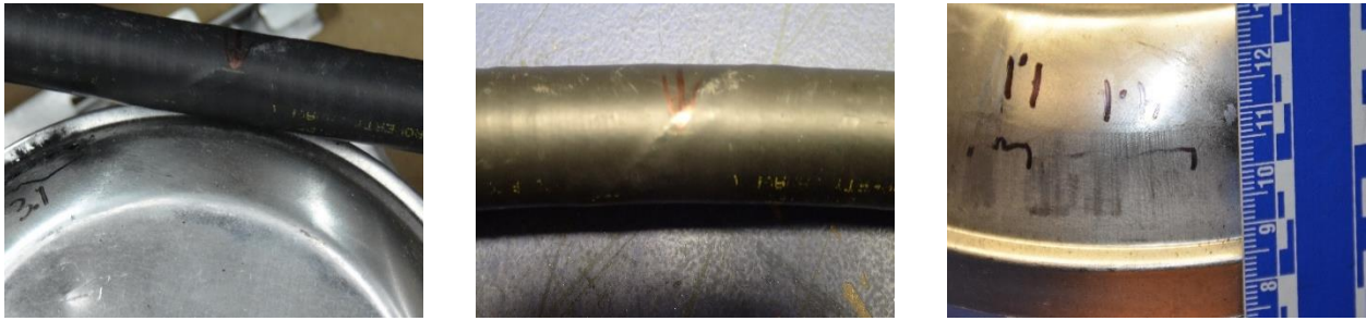
Figure 43 Test 4.1 in place (left). Undamaged FlashShield™ (center) and light fixture (right) post-test.
