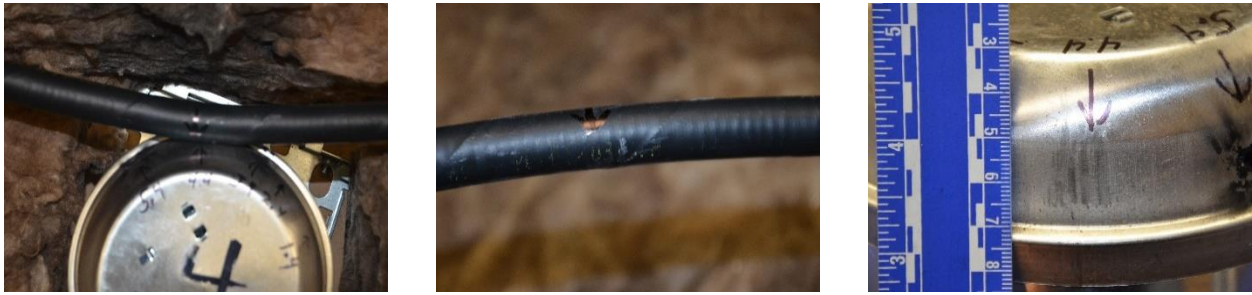
Figure 46 Test 4.4 in place (left). Undamaged FlashShield™ CSST (center) & light fixture (right) post-test.
