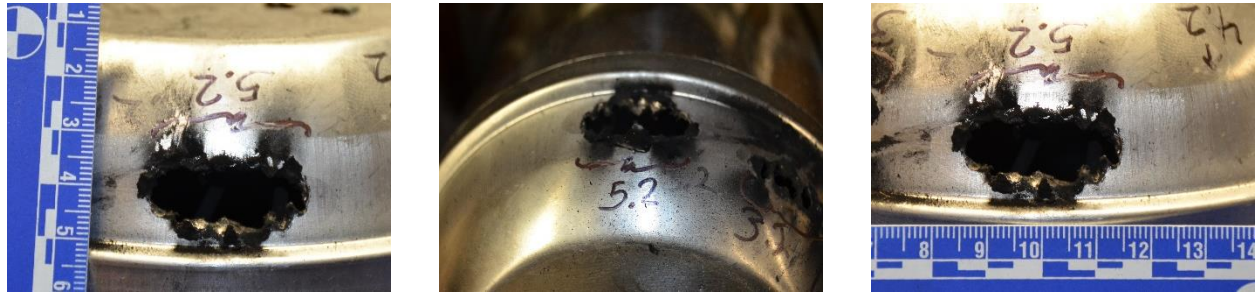
Figure 55 Damage to light fixture in test 5.2.
