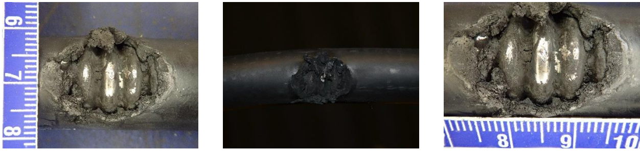
Figure 39 Damage to CounterStrike® CSST in test 3.5.
