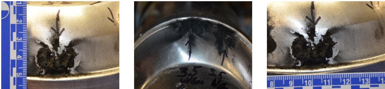
Figure 40 Damage to light fixture in test 3.5.
