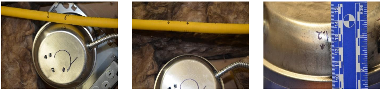
Figure 13 Test 1.2 in place (left). Undamaged WARDFlex® (center) and light fixture (right) post-test.
